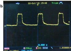
a) Set up of the pulse on the digital display, b) corresponding microwave output measurement
