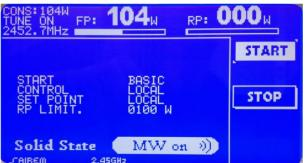
All operating parameters and control status, as well as any possible fault, forward power and reflected power are displayed on the screen. The forward power set-point is pre-displayed before starting.
